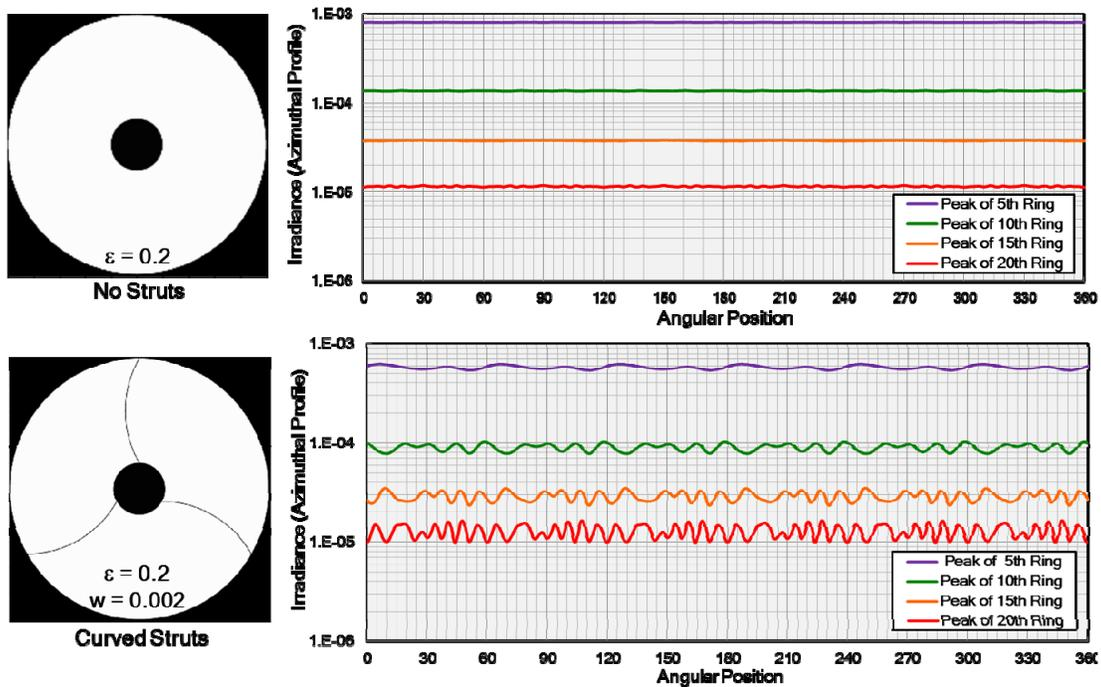
Figure 17. The azimuthal irradiance profiles are indicated at the peak of the 5<sup>th</sup> diffraction ring, as well as the 10<sup>th</sup>, 15<sup>th</sup> and 20<sup>th</sup> ring, thus spanning the habitable zone for exoplanets.
