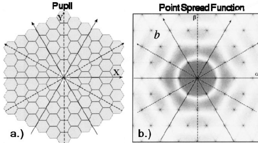
Figure 2. a.) Close-packed hexagonally segmented mirror with segmentation order  $M = 5$  consisting of  $N = 90$  segments, solid and dashed arrows illustrate the double  $\pi/3$  symmetry of the system ; b.) predicted diffraction peaks that populate the image field exhibit the same  $\pi/3$  symmetry as the pupil plane.
