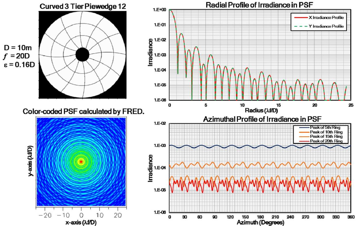
Figure 18. The 3 Tier Piewedge 12 segmented mirror configuration is illustrated with a relative gap width of  $w = 0.002D$ . The simulated PSF is devoid of any discrete narrow diffraction flares; however, substantial interference effects are apparent. The x and y-axis radial irradiance profiles and several azimuthal irradiance profiles are also indicated.
