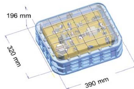
Fig.6. MERLIN laser housing
