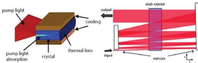
Fig.5. Left: InnoSlab concept; right: amplifier beam path
