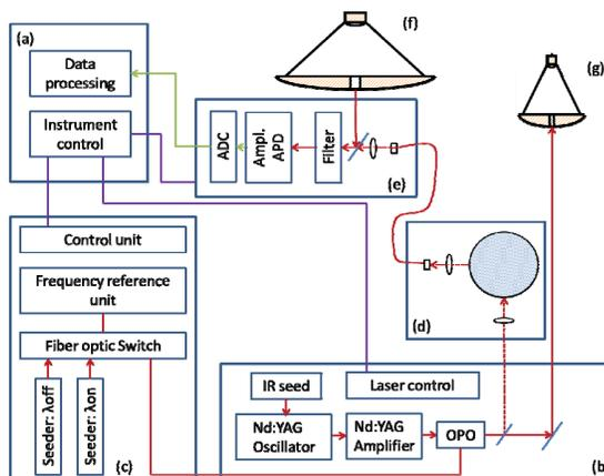
Fig. 4. Instrument setup: (a) instrument control unit, (b) laser, (c) frequency reference, (d) energy calibration, (e) receiver, (f) Rx telescope, (g) Tx optics
