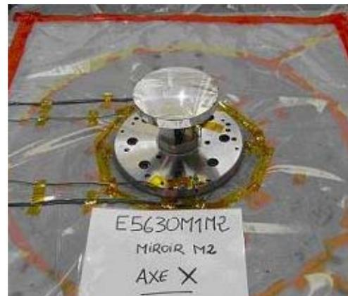
Fig. 9: M2 during vibration tests
