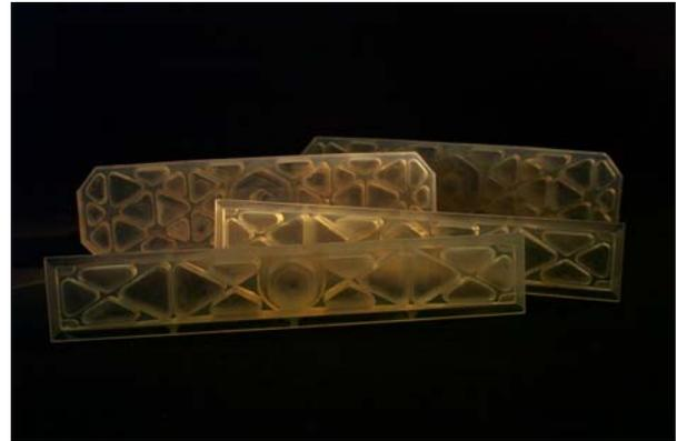
Fig. 8: M3 and MR mirrors (M1 and FM2) before coating
