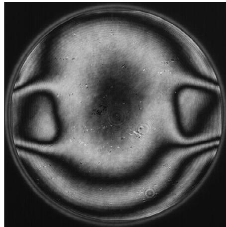
Fig. 8: Interferogram and surface after insert bonding
