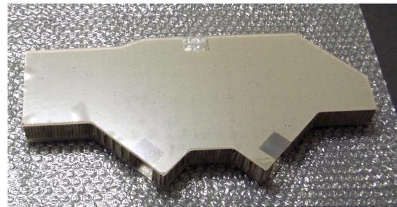
Fig. 2 Picture of the Base-plate built for the Aladin Mie Spectrometer
