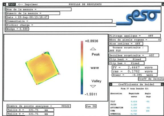
Fig. 10: Interferogram of the polished sample including edge effects
