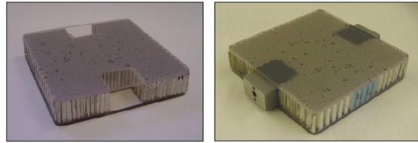
Fig. 6: Zerodur sandwich sample before and after bonding the inserts
