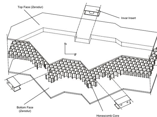
Fig. 3 Exploded view of the Base-plate built for the Aladin Mie Spectrometer
