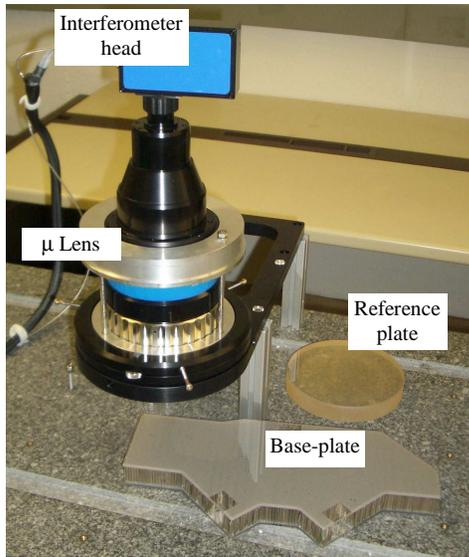
Fig. 4 Set-up for interferometric verification of the base-plate
