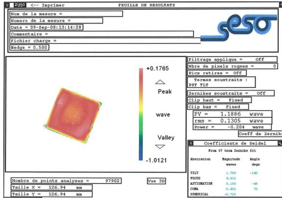
Fig. 9: Interferogram of the polished sample removing edge effects
