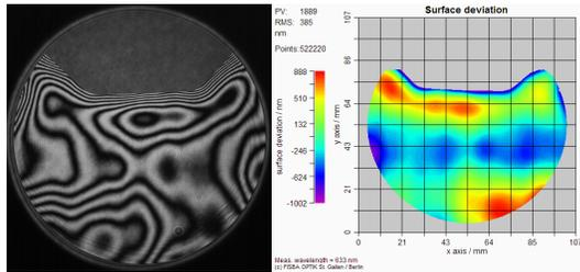
Fig. 5 Example of interferometric measurement of the base-plate surface
