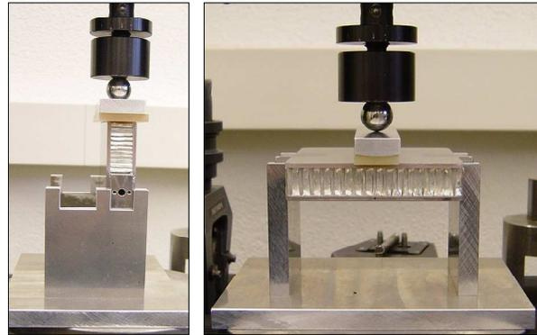
Fig. 7: Baseplate insert shear and bending strength test setup
