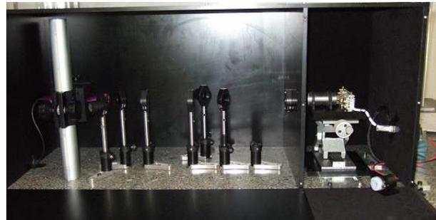
Fig. 8. Photomultiplier calibration bench
