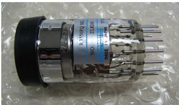
Fig. 7. PHEBUS NUV photomultiplier
