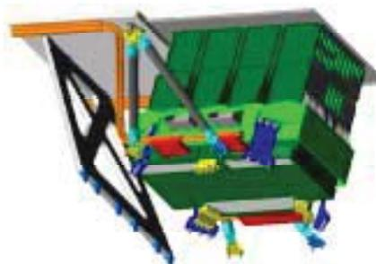
Fig. 18. View of the Pléiades SEDHI (including the focal plane and the radiators)
