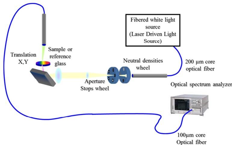
Fig. 2. Spectral uniformity measurements set up.
