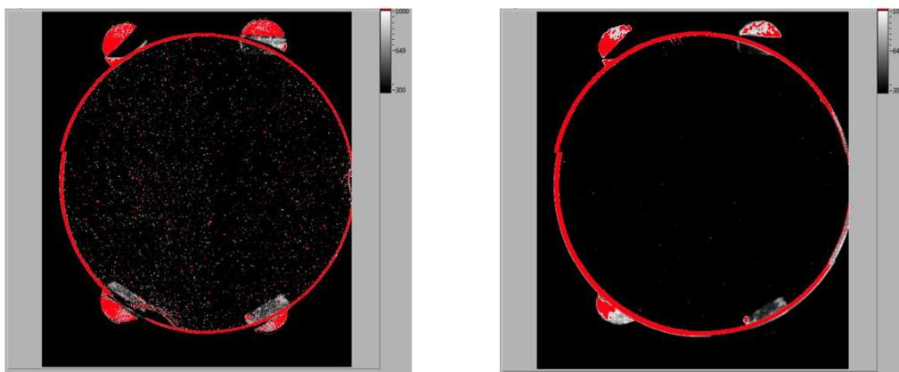
**Fig. 9.** Cosmetics measurement on the filter side of the VIS Filter 3 (before and after optimization of the cleaning procedure of the deposition machine).
