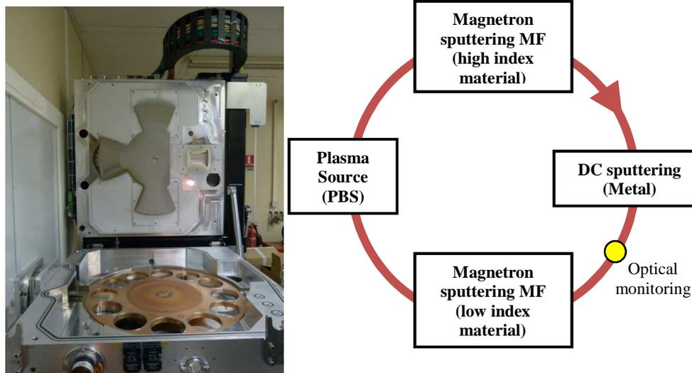
Fig. 1. HELIOS deposition process chamber.
