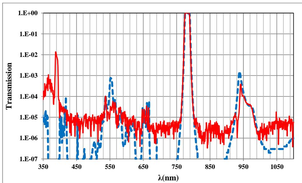
**Fig. 7.** Comparison between theoretical (dashed line) and experimental (solid line) transmission of the VIS Filter 2 in logarithmic scale.
