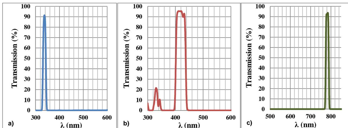
Fig. 4. Transmission spectra of the UV-VIS deposited filters: UV Filter (a), VIS Filter 1 (b) and VIS Filter 2 (c).
