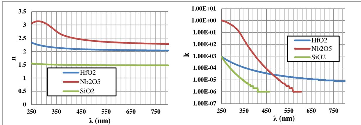
Fig. 3. Refractive indices ( $n$ ) and extinction coefficients ( $k$ ) of the materials deposited with the HELIOS System.
