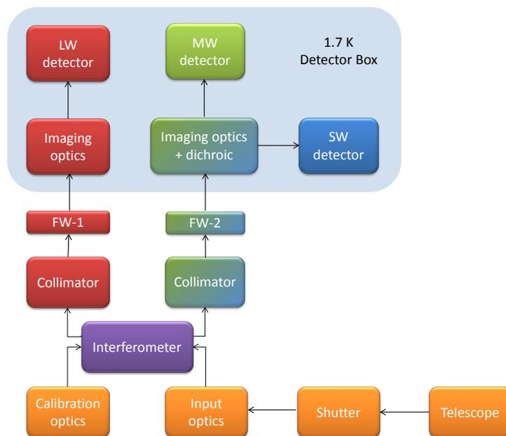
Fig. 1. System block diagram of the Safari instrument.
