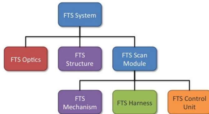
**Fig. 6.** Block diagram of the FTS system.
