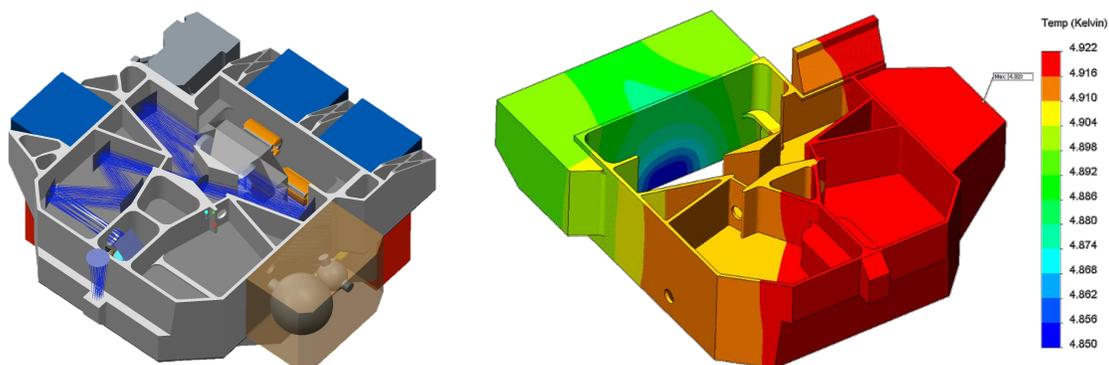
Fig. 5. Design of light-tight compartments and result of thermal analysis.
