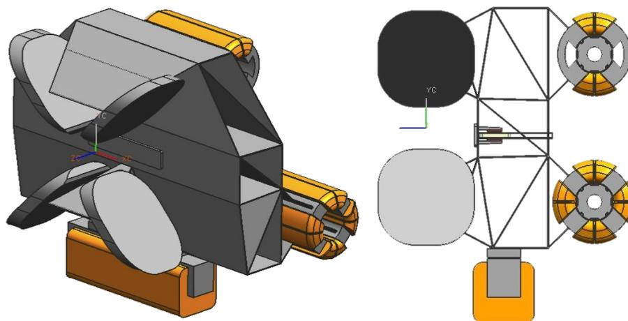
**Fig. 7** Scan mechanism concept for the Safari FTS based on magnetic bearings [9-11].
