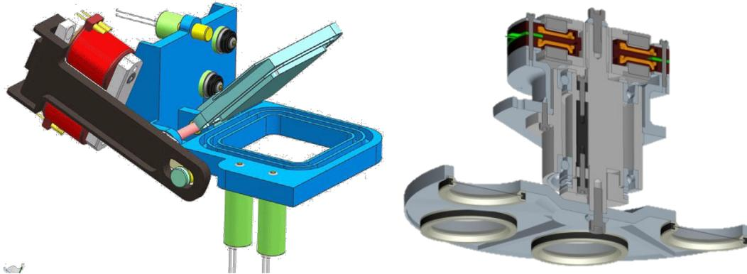
Fig. 2. Shutter mechanism concept (left) and Filter Wheel mechanism concept (right) for Safari.
