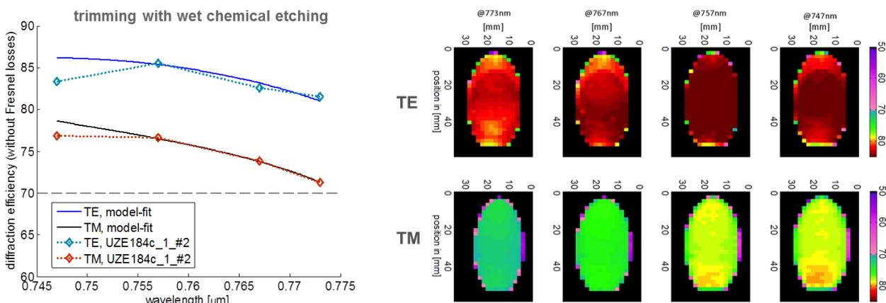
**Fig. 4:** a) Left: Predicted and measured diffraction efficiency of a NIR PG+P grating for two polarization directions. The resulting polarisation sensitivity is below 7%. b) Right: Homogeneity of efficiency across the pupil
