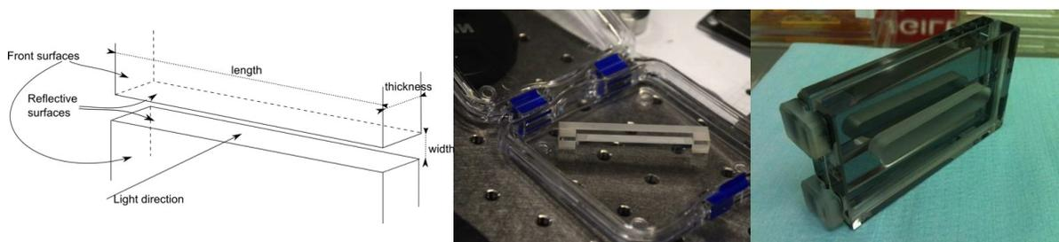
**Fig. 5:** a) Left: General setup of a slit homogenizer (SH). b) Middle: SH prototype for Concept A (photo courtesy of Airbus DS) c) Right: SH prototype for Concept B (photo courtesy of WinLight)
