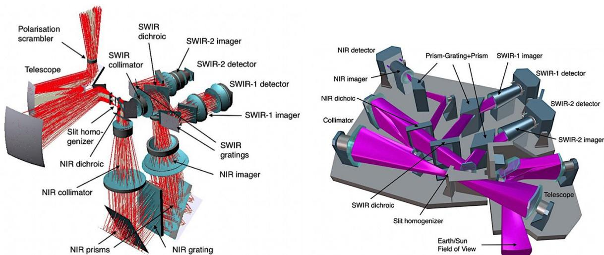
**Fig. 1:** Designs concepts for the CarbonSat instrument resulting from the industrial Phase A/B1 studies. Concept A on the left was developed by the consortium led by Airbus DS, Concept B on the right by OHB/Thales.
