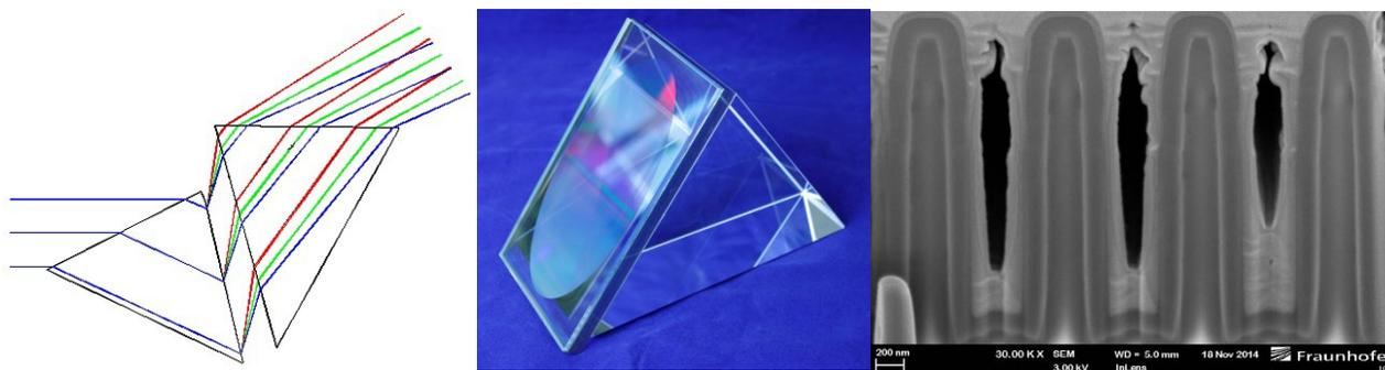
**Fig. 3:** a) Left: Light path through the prism-grating-prism (PG+P) assembly. b) Middle: The bonded prism grating prototype assembly (photo courtesy of IOF). c) Right: SEM image of the binary sub-micron structure on the surface of the grating substrate.
