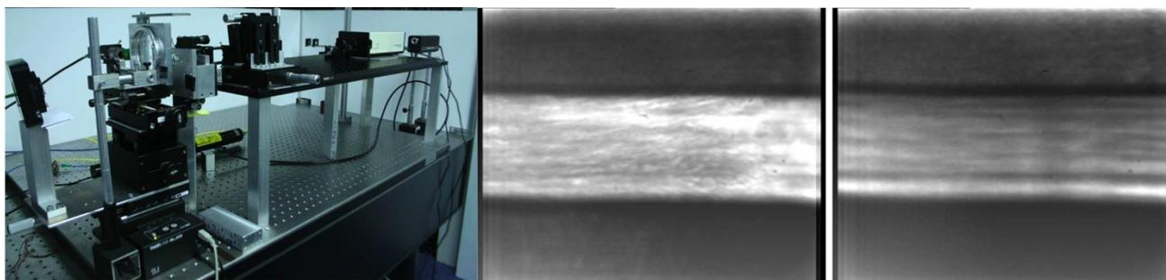
**Fig. 6:** a) Left: Test setup for SH performance testing (photo courtesy of ITO). b) Middle: SH response (image of slit exit) to homogeneous illumination. c) Right: SH response to half-slit (knife-edge) illumination.
