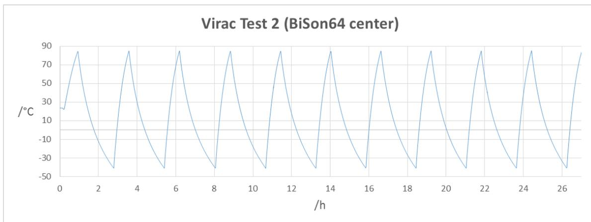
Figure 3. Typical thermal cycling profile used for BiSon64 sensors.
