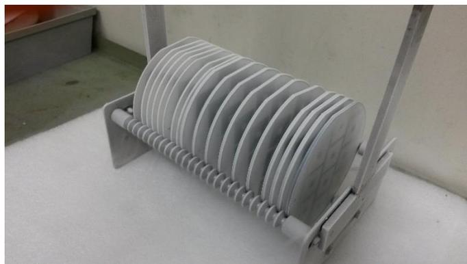
**Photo 2.** Wafers after liquid nitrogen dipping
