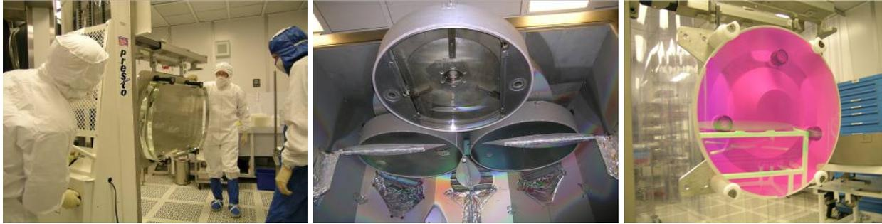
Figure 8. Optics Support Facility. (Left) Handling of a truncated 94 cm fold mirror. (Middle) Interior of the coating chamber during the coating of a truncated 94 cm fold mirror. (Right) Final product for a 75 cm HR coating (200 lb weight).
