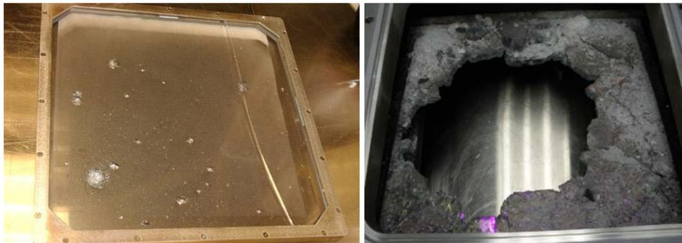
Figure 7. Used Debris Shields. (Left) Moderate damage on Z shot consisting of several shrapnel sites and “soot” coating. (Right) Severe damage during a Z shot.
