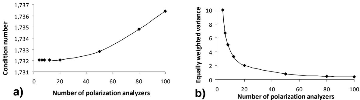
Fig. 7. Analysis of the *CN* (a) and *EWV* (b) as a function of the polarization analyzers number
