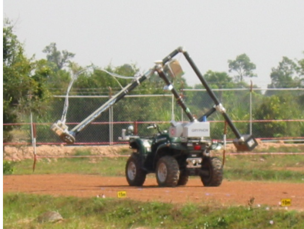
Figure 4. ALIS mounted on a buggy Gryphon (developed by Tokyo Institute Technology). A Vivaldi antenna is attached with a metal detector sensor on the robot arm. The buggy mounted ALIS uses a VNA based GPR for the best performance.
