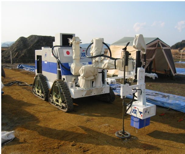
Figure. 2. SAR-GPR mounted on Mine Hunter Vehicle.
