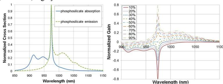
Fig. 1, from left to right, cross sections and gain spectra of phosphosilicate fibers at various inversions.
