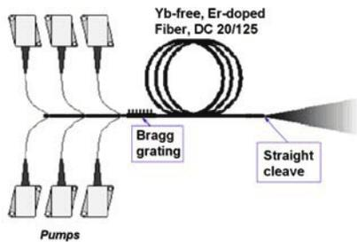
**Figure 1.** Optical layout of the resonantly cladding-pumped fiber laser based on Liekki Er60-20/125 DC fiber pumped at 1532.5 nm.
