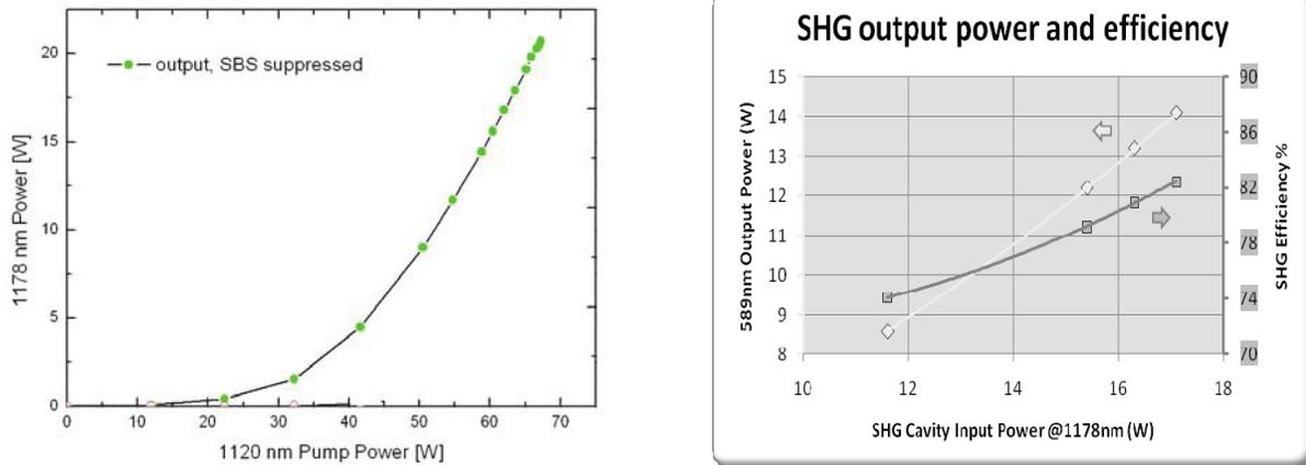
Fig. 1 Left: output power of the 1178nm fiber Raman amplifier as a function of pump power;
