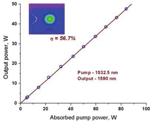
**Figure 2.** Output versus absorbed pump power dependence obtained for the resonantly cladding-pumped Er-doped FBG-laser shown in Fig.1.
