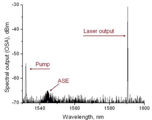
**Figure 3.** Spectral output of the FBG laser shown in Fig.1 (ANDO AQ6370 optical spectrum analyzer, resolution 0.05 nm).
