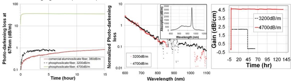
Fig. 2, from left to right, measured PD loss, PD spectra and gain versus time. Inset is absorption spectrum.
