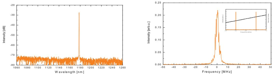
Fig. 2 Spectrum of the amplifier output. left) a broad range spectrum taken with an Ando spectral analyzer showing 40 dB contrast; right) a detailed spectrum of the 3.5MHz line taken with a Fabry-Perot interferometer (1 GHz FSR).
