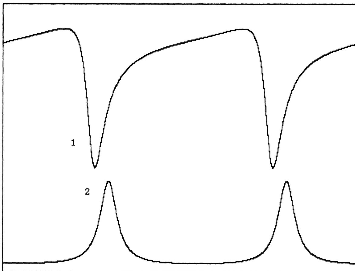
Fig.6. Computer simulated Fabry-Perot reflection (1) and transmission (2) spectra. Absorption coefficient  $a=0.13$ ,  $R_1$  and  $R_2$  phase difference  $f=0.6$ .
