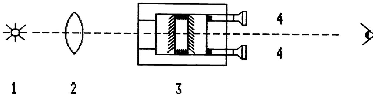
Fig.1. Set up for Fabry-Perot etalon adjustment.
