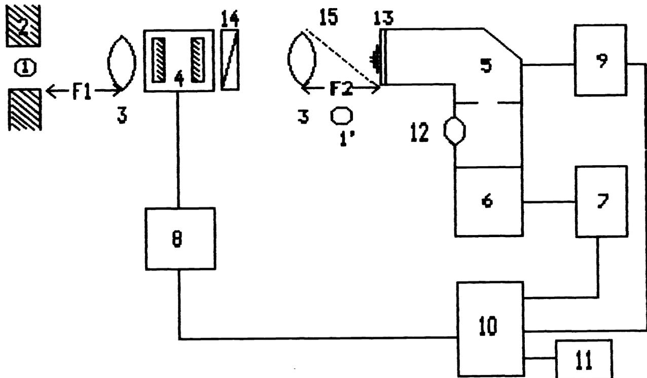
Fig.2. Spectral installation with Fabry-Perot etalon.
