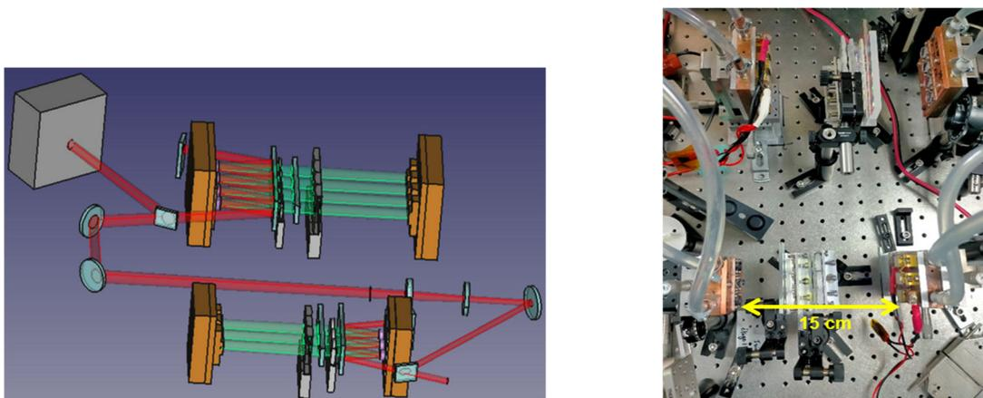
Figure 4: 3D layout and laboratory set-up picture of the 400-mJ amplifier.
