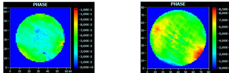
Figure 5: Wavefront measurement (with Phasics SID4 sensor and software) of a plane wave after reflection through a pumped functionalized Nd:YAG disk. Left: stage 1 disk. Right: Stage 2 disk.
