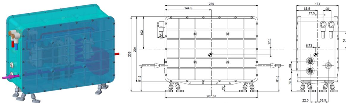
Figure 8: CAD drawing of the elegant breadboard, with main dimensions
