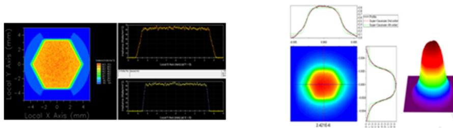
Figure 3: Pump distribution at the disk. Left: simulated in FRED® software. Right: Measured with Ophir-Spiricon beam profiler.
