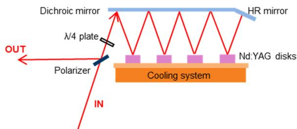
Figure 1: Amplification module based on active mirror technology.
