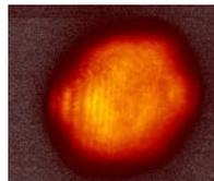
Figure 6: Output beam distribution at 400 mJ, 50 Hz.
