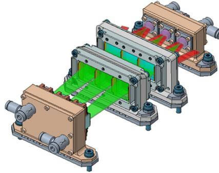
Figure 7: Optomechanical design of amplifier stage 1
