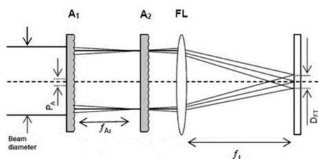
Figure 2: Flat-top illumination using microlens arrays.
