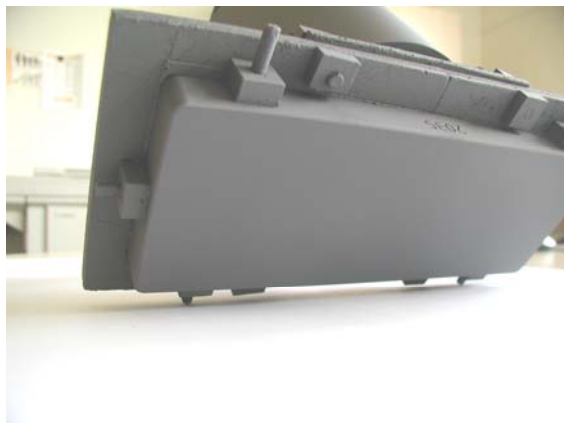
Fig. 1. Baffling of M4 viewed after CVD deposition
