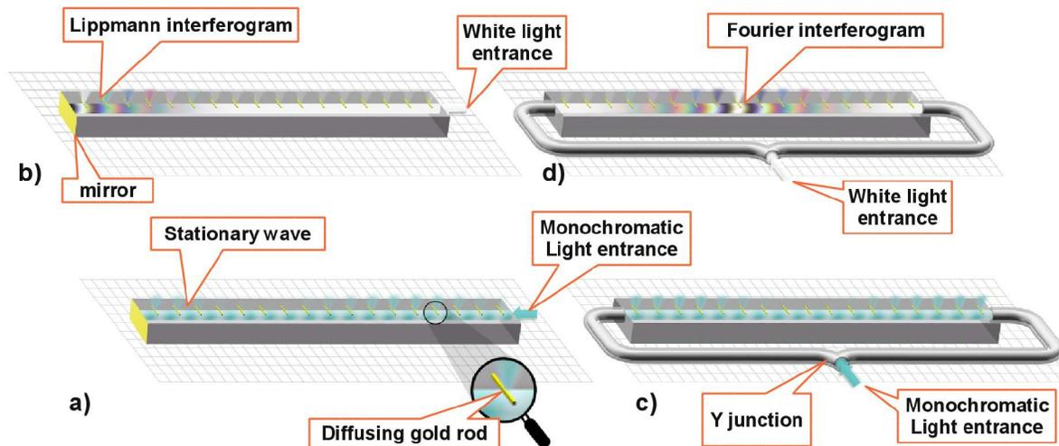
**Fig. 1.** SWIFTS principles Nanodetectors are placed in the evanescent field of the waveguide. Each detector samples a small part of the flux over a distance smaller than the fringe size. For polychromatic input light, the resulting superimposition of stationary waves lead on to a Fourier interferogram sampled by the set of nanodetectors. The lower 3D artist views present the corresponding SWIFTS devices for colored entrance light and the resulting interferograms.
