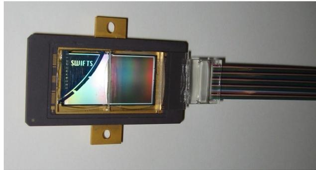
**Fig. 3.** SWIFTS 400-1000 mockup: A 1K frame transfer CCD is surrounded by a glass plate containing parallel waveguides and diffusing dots is fed by optical fiber bundle. A  $0.2\text{cm}^{-1}$  apodized spectral resolution is foreseen.
