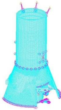
**Fig. 5.** Telescope finite element model
