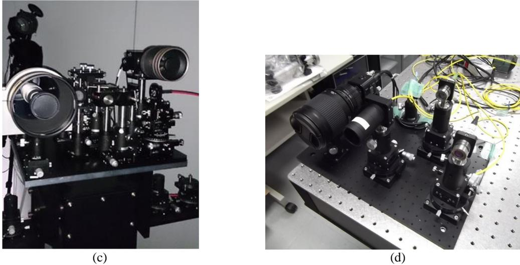
Fig. 3. Photo of the optical system setup: c. receiver module; d. transmitter module
