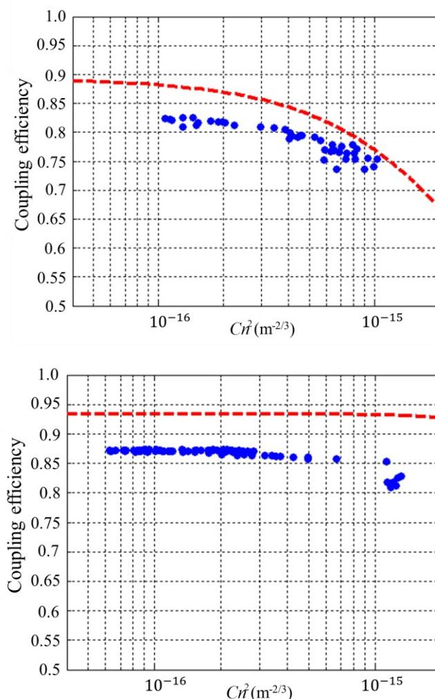
Fig. 6. The coupling efficiency of laser beam to MMF
