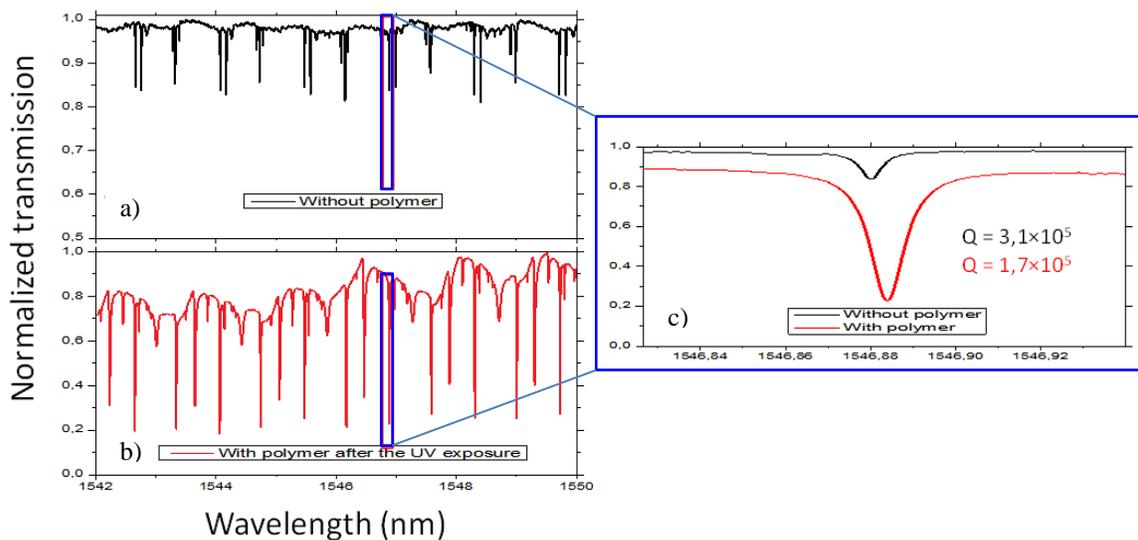
**Fig.4.** Spectral transmission of a SiO<sub>2</sub> microdisk before a) and after b) the polymer encapsulation, c) zoom on a resonance peak
