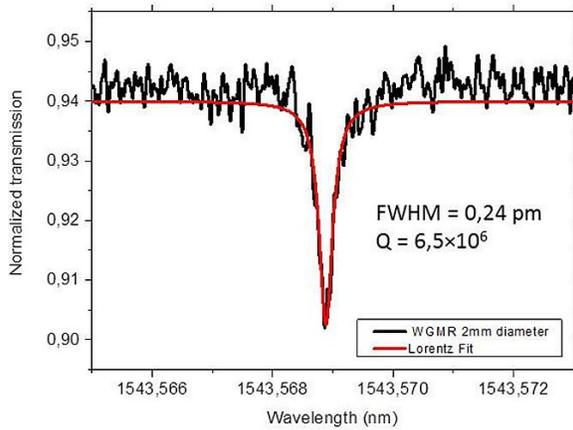
**Fig. 3.** Spectral response of a 2 mm diameter SiO<sub>2</sub> microdisk realized with the optimized process flow
