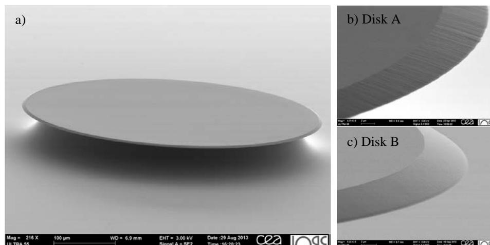
**Fig.1.** a) SEM picture of a 400 μm diameter SiO<sub>2</sub> microdisk; b) Disk A - roughness of a disk edge interface with standard fabrication process without roughness optimization steps; c) Disk B - roughness interface with specific process steps inspired from the Vahala group [10]
