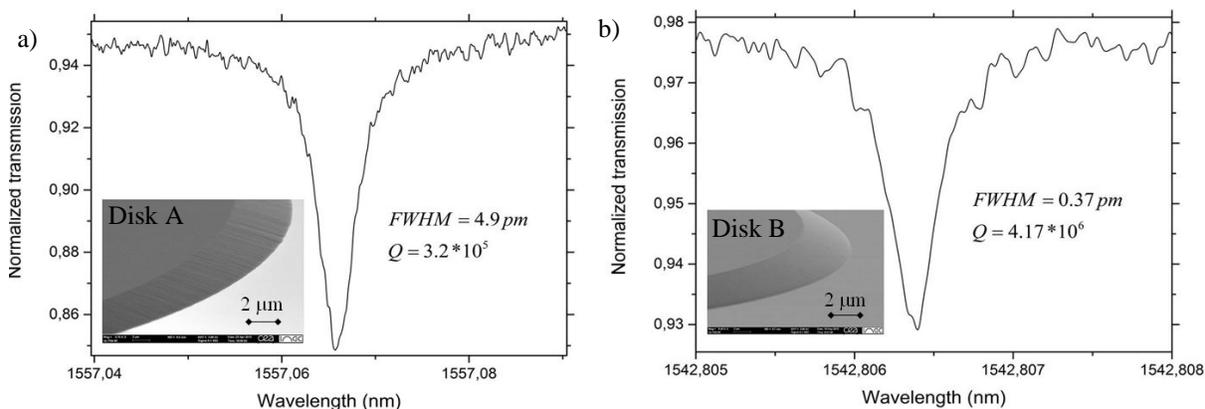
**Fig.2.** Transmission spectra across a WGM resonance for a) non optimized process on disk A b) roughness optimized fabrication process on disk B
