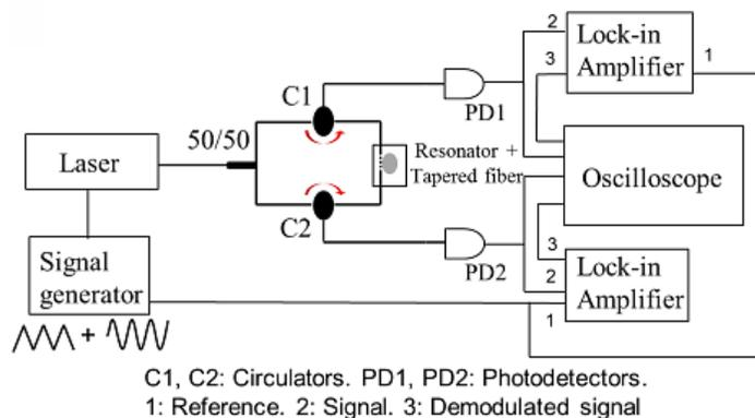
Fig.5. First system test setup
