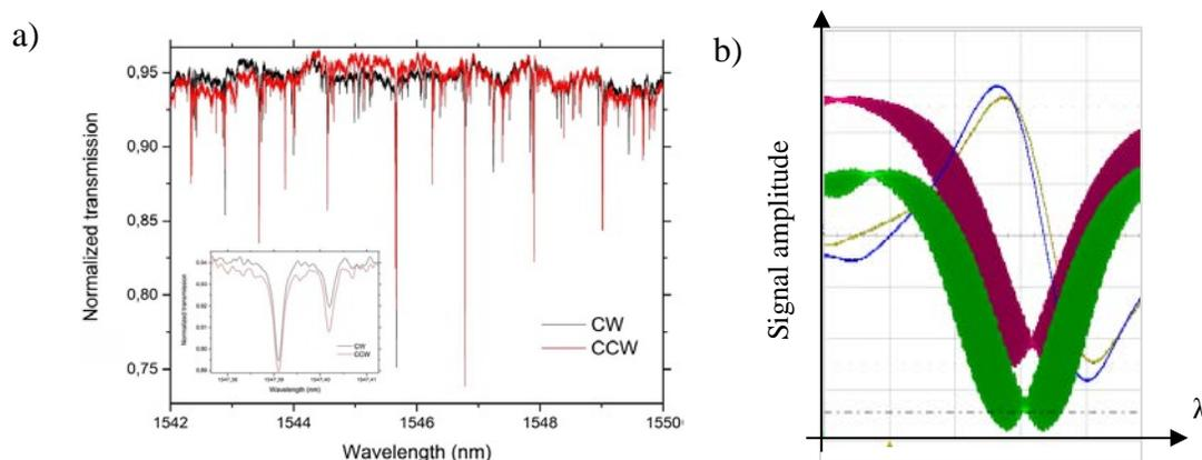
Fig.6. a) The WGMR spectral response on 8 nm range scan for CW (black) and CCW (red) lightwaves. The inset is a zoom for the peaks at 1547.39 nm. b) Resonant peaks (green and magenta) and their respective demodulated signals (blue and yellow) over 50 pm scan for the CW and CCW excitations.
