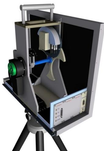
**Fig. 2.** The DFU carousel inside the filter radiometer housing, the cover of which has been removed for easy viewing. In the picture, only one DFU is mounted. In total the filter radiometer can hold three DFUs, for UV-VIS, NIR and SWIR.
