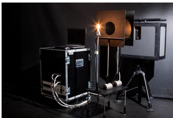
**Fig. 3.** Photograph of the complete system, set up to measure the spectral irradiance of a FEL lamp. From front to back: electronics box with controlling laptop, FEL lamp, external baffles to shield for stray light and filter radiometer.
