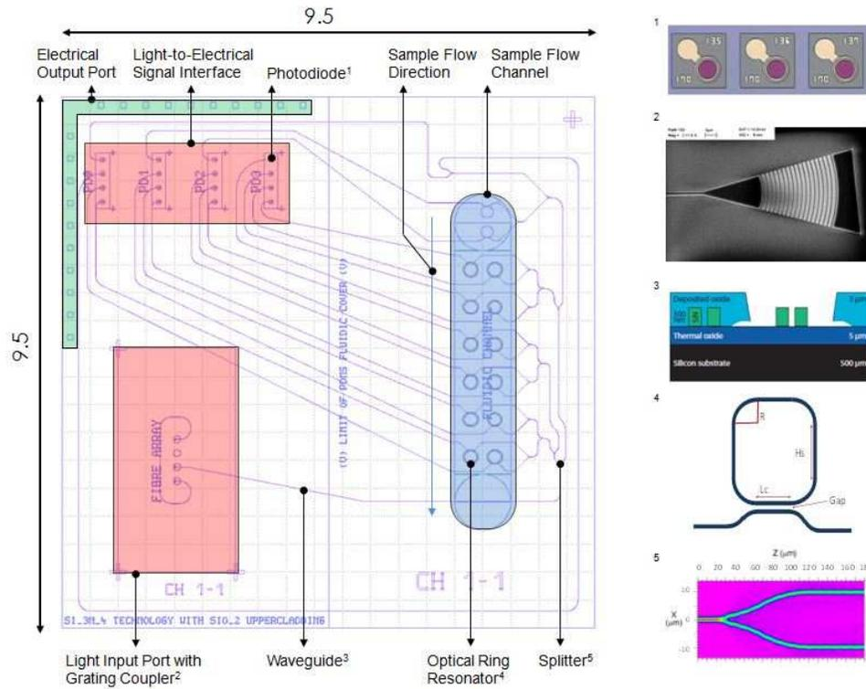
**Fig. 4** Design of the photonic integrated circuit (PIC) with outer dimensions and functional sub-systems. The functional sub-systems are shown on the right in a detailed view.
