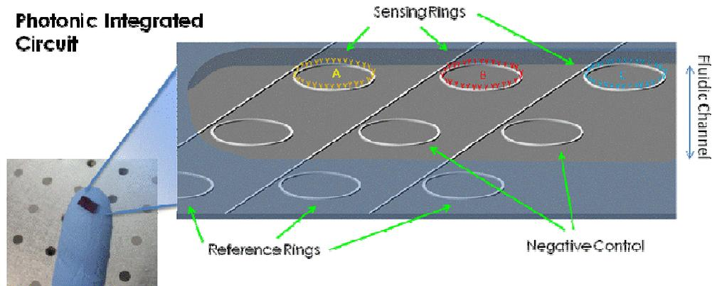
Fig. 3 Picture of the photonic transducer. Left: General view of a PIC device. Right: Detail of resonating structures (Ring resonators with radius  $\sim 100\mu\text{m}$ ) used in the detection. In each circuit three rings are shown: one to compensate derivatives other for the negative control of the detection and a third one for the measurement. The molecular bioreceptors are represented in different colours to illustrate the multiple target capabilities of the technology.
