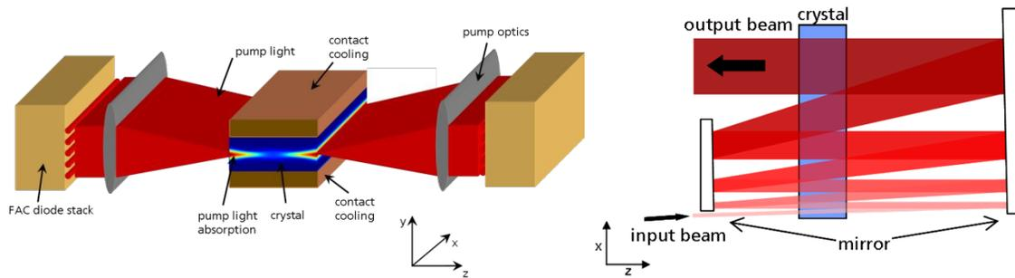
Fig. 3. Schematic of InnoSlab Pump configuration (left) and folded signal beam path (right)
