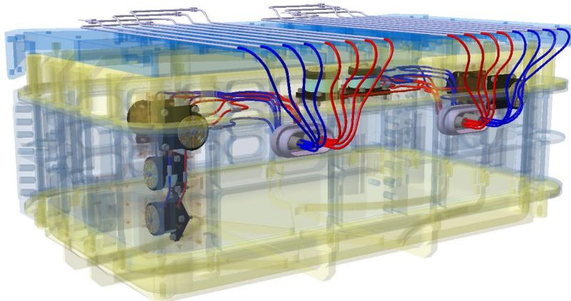
Fig. 2. Housing with LHP – Thermal management Sub-System
