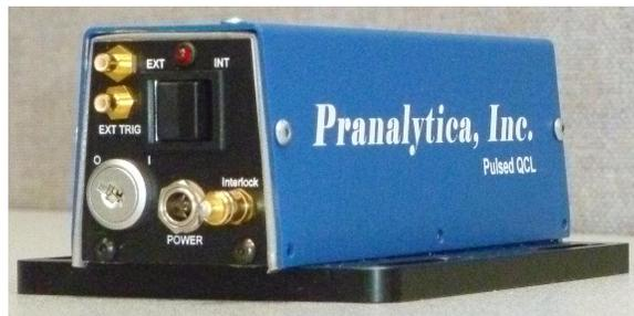
**Figure 2. Packaged QCW operation QCL of Figure 1, including rechargeable batteries, weighs less than 450 g (<16 Oz) and produces >3.5 W of average power at a wavelength of ~4.6  $\mu\text{m}$ .**
