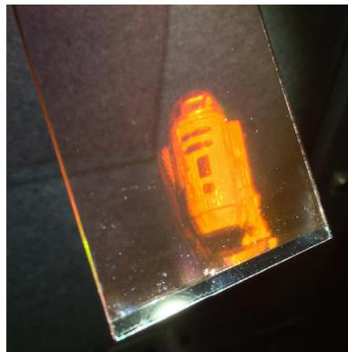
Fig. 4. Holographic image illuminated by white light
