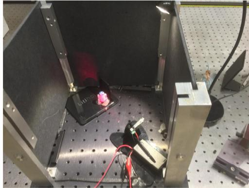
Fig. 2. Configuration used for one-minute exposure reflection hologram viewable with white light illumination—one side and cover removed.
