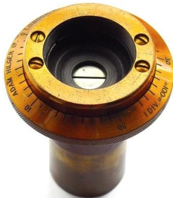
Figure 10. The symmetrical slit.
