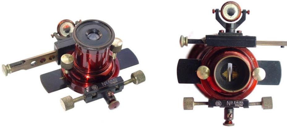
Figure 7. The shutter eyepiece.
