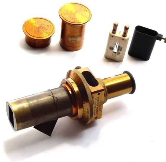
Figure 8. The symmetrical slit mount, with a recess in a block into which the thermopile fits.
