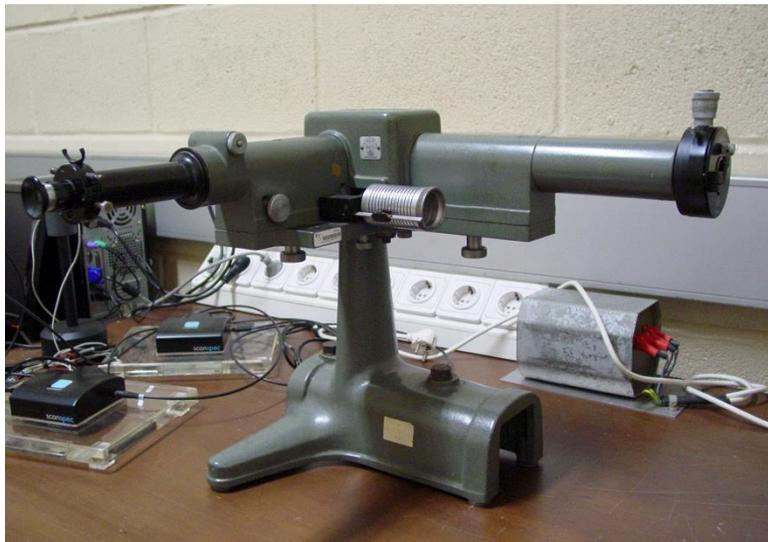
Figure 17. The 1964 Hilger & Watts spectrometer together with two computer connected CCD spectrometers in the Optics teaching laboratory of the Physics and Astronomy Department, Faculty of Science (May 2015).
