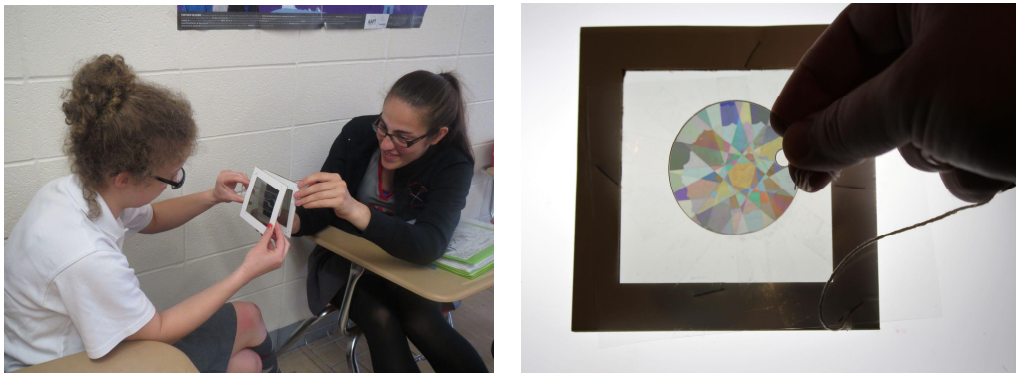
Figure 5. Students examine a stressed plastic "U" shape between crossed polarizers (left); A completed "art" project (right)
