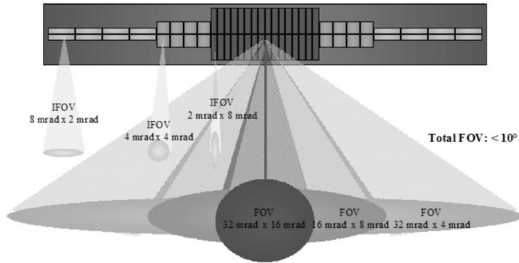
Figure 12. Block Scheme for improving single sub-pixel element resolution in large area signal extraction.
