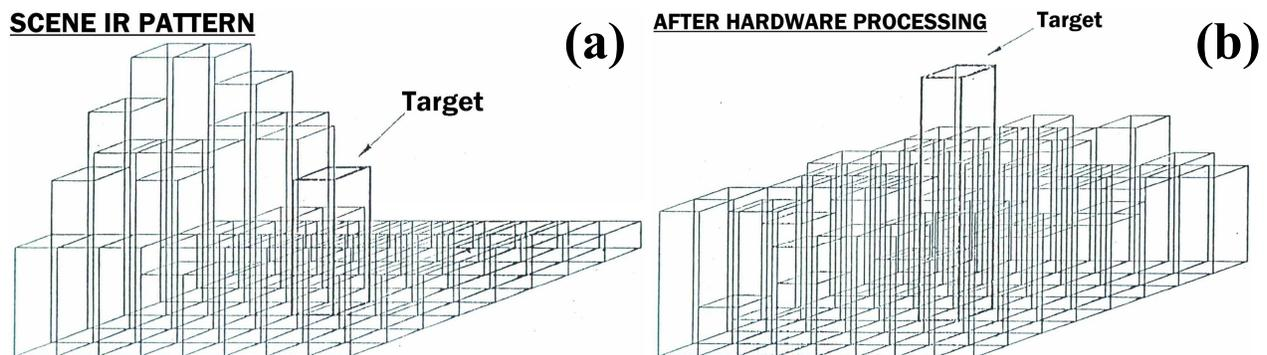
Figure 10. (a) Point Source Target Signal Immersed in High Intensity Clutter [7] and (b) Point Source Target Signal Enhanced by Smart Sensor Integrated Extraction [7].
