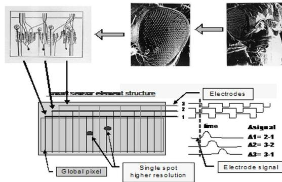
Figure 5. Smart Sensor emulating Fly-Eye recognition structure with an integrated 3 electrodes modulation [19, 20, 21].
