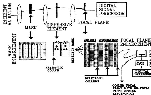
Figure 4. Multispectral reticule structured sensor.
