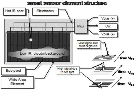
Figure 6. Detection of Point Source Target in presence of high clutter unwanted signals with increased resolution obtained by a 3 differential electrodes: This 3 electrodes structure was repeated 8 times within large area 1024 FPAs sensor elements.
