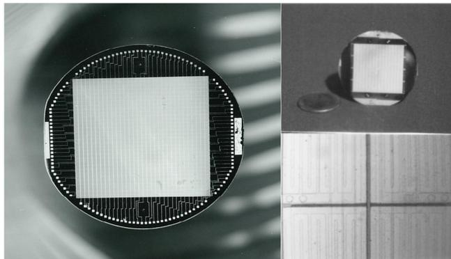
Figure 8. IR FPAs (1024 sensors, each one with 3x8 sub-pixels) Electronica Spa Rome -Italy 1976.
