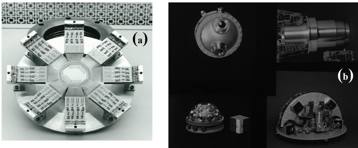
Figure 9. (a) IRWR TARSIO (Tactical Infrared System Omnidirectional) MLAW Airborne Warning and Alarm System (b) CERBERO Infrared Surveillance Alarm and Warning System  $2\pi$  Navy System, Electronica S p a Rome -Italy (1980).
