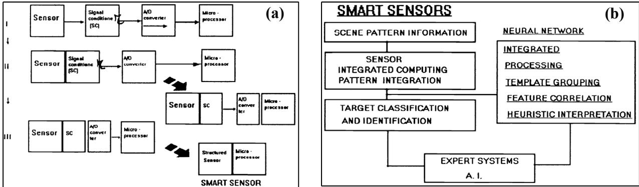
Figure 2. Sensor structure evolution (a) and smart sensor functions (b) [9][19].
