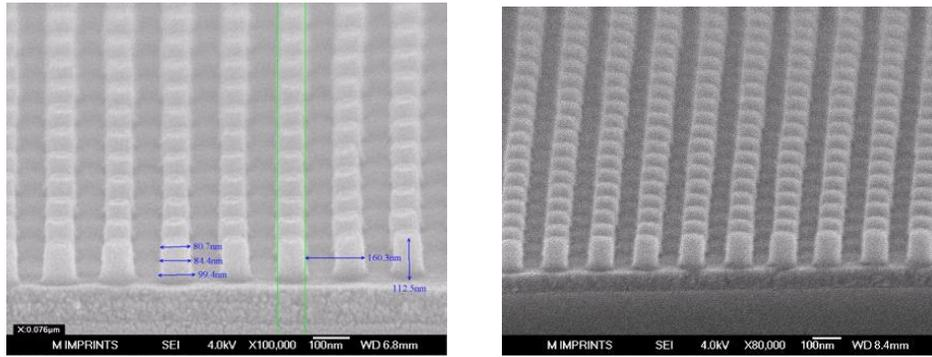
Figure 5: Template replication results. Left hand micrograph shows imprinted features from the ebeam master template, the right hand micrograph shows imprinted features from the replicated template
