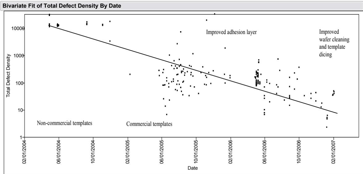
Figure 9: Defect improvement over time for SFIL.(from ref 21)
