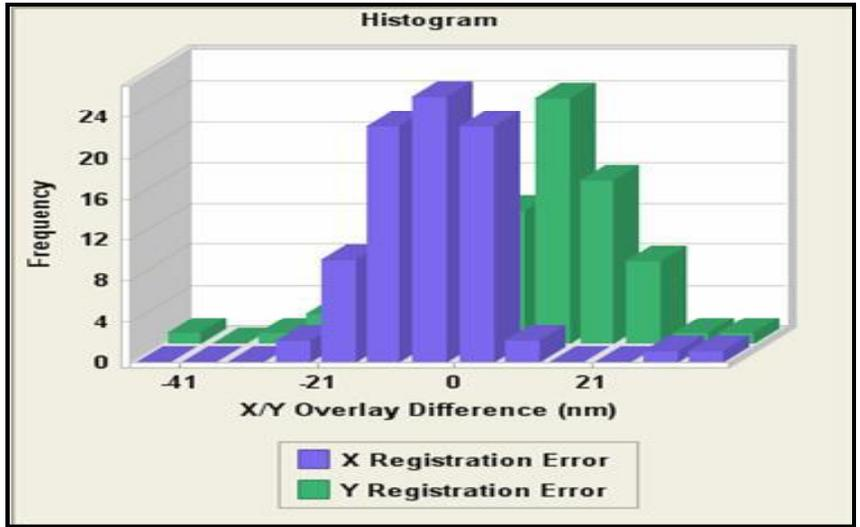
Figure 8: Overlay data from imprint patterns over 193nm optically exposed underlayers. 32 fields per wafer and 81 locations per field (from ref 20)
