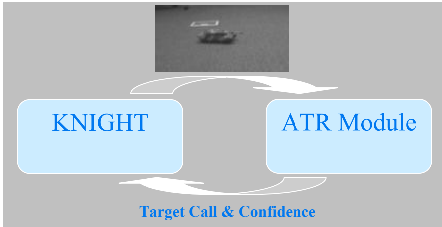
Figure 7: ATR – Tracker interactions occur only at each client. The results of the ATR including class label and confidence are sent to the server.
