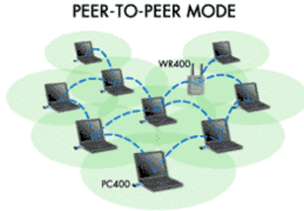
Figure 6: Example of a ad-hoc Peer-to-Peer network.
