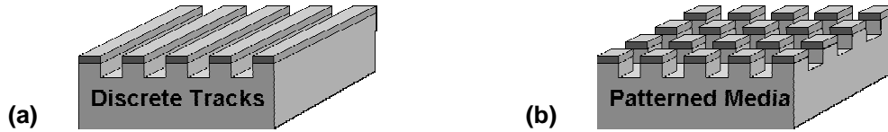
Fig. 11. Schematics of (a) Discrete Track media and (b) Patterned Media. In Discrete Track media, only the tracks on the disk are patterned lithographically, while the bit transitions along the track continue to be defined by the thin-film head during recording. In fully patterned media, both bit dimensions on the disk are defined lithographically.
