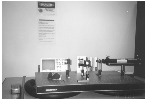
Fig. 7: Each mini-lab is typically equipped with a laser, an oscilloscope, vibration-isolated breadboard, goggles, flashlights, lamps, screens and assorted hardware. The precision optics and detectors are kept in a humidifier cabinet when not in use.
