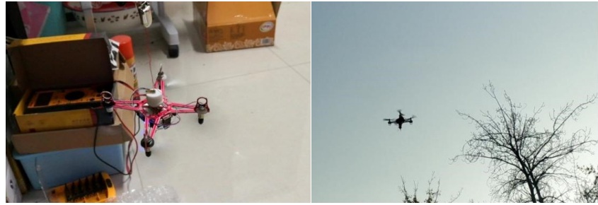
(a) Learning mode: hanged by a string (b) Testing mode: flying and fine-tuning
