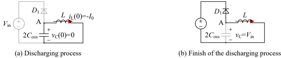
Figure 4. Equivalent circuit example of the ZVS process at the dead time instant of t_0 .
