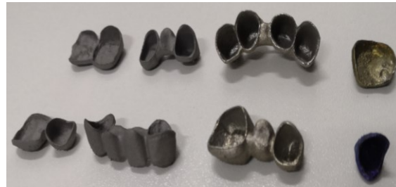
Figure 8. The denture model made by laser rapid manufacturing technology.
