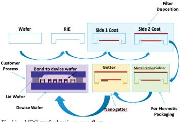
Fig 11 - MBO wafer level process flow.
