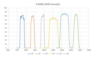
Fig 10 - Measured results from a MBO 6 band LWIR assembly
