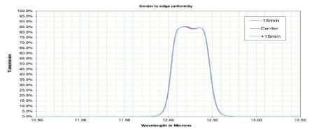
Fig 9 - Uniformity over 30mm dia
