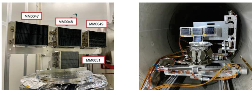
Figure 1. Photographs showing all four SPO mirror modules mounted in the holder as seen from the detector side. (left) In the image the mirror modules are labeled. (right) shows the final setup inside the PANTER beamline tube of the optics in their holder mounted on the hexapod which itself is mounted upon a translation stage. The movable mask for selecting the MM or XOU to be studied can be seen located behind the optic holder.
