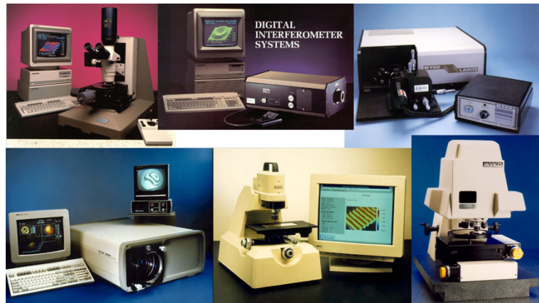
Fig. 10. (top) Early Wyko product line based upon HP Workstations: Topo, Sirus, and Ladite. (bottom) Wyko products from 1990's using PCs: 6000, RST, and NT2000. (Photos courtesy of Jim Wyant).
