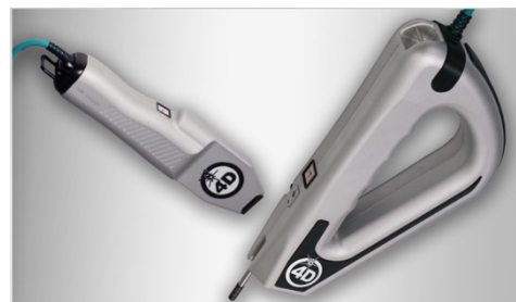
Fig. 21. 4D Inspec, a handheld vibration-immune metrology system for quantification of fine-scale features in manufacturing environments [18].
