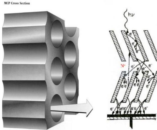
Figure 1. Schematic showing mode-of-operation of the MCP<sup>3</sup>
