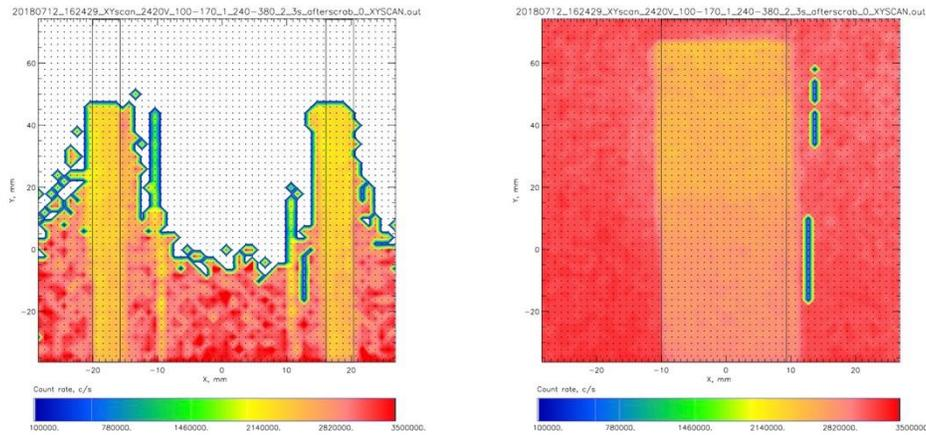
Figure 9. Gain distribution measured over the START sectors (left picture) and over the STOP sector (right picture). The START sectors consist of two parts “anode1 (left side)” and “anode1 (right side)”. The STOP sector comprises one part “anode2 (center)”. Vertical rectangles define the integration bands used to calculate the gain profiles.
