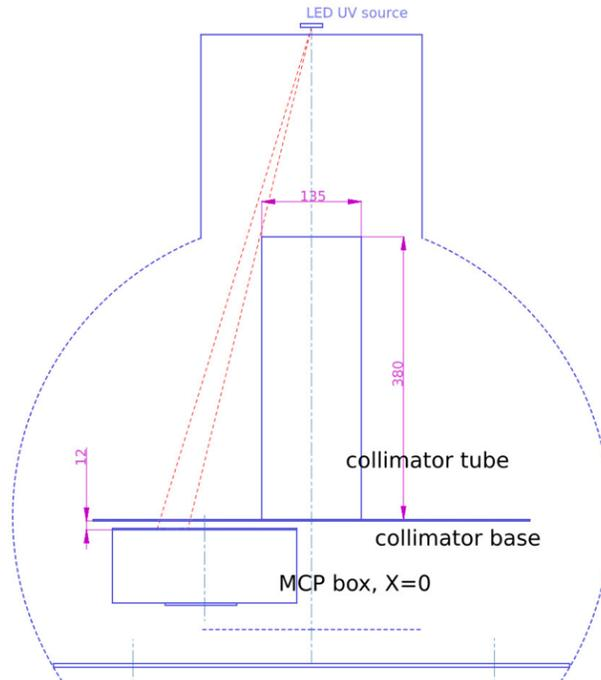
Figure 3. The experimental setup allows two configurations. In the Scrubbing and Charge accumulation configuration the MCP setup is exposed to UV emission. In the Differential Gain characterization configuration the MCP box is located below the collimator tube. The needle UV beam is used to measure the MCP gain step-by-step in every point of the MCP surface. The small plate shown under the MCP box is a XY stage interface.
