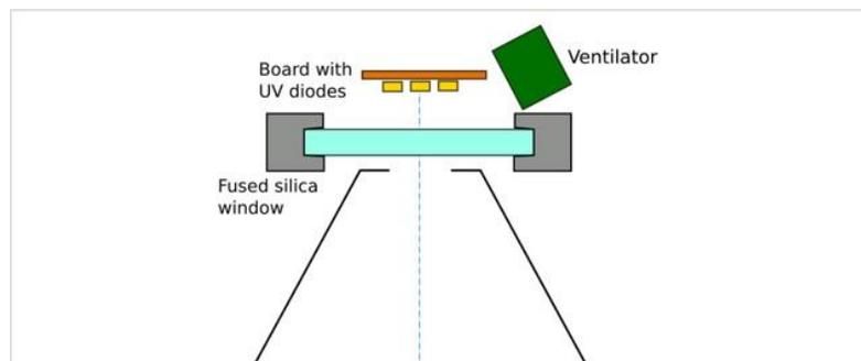
Figure 4. UV LED source installation. The UV source is located outside the vacuum chamber to allow better cooling of the powerful UV LEDs by means of a ventilator. UV light emitted by the UV LEDs passes through a fused silica window which is transparent to UV emission.
