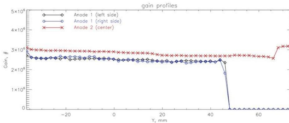
Figure 10. Gain profiles shown for the START sectors: black line - “anode1 (left side)”, blue line - “anode1 (right side)” and for the STOP sector: red line - “anode2 (center)”. The gain profiles are integrated over the vertical rectangles shown in the gain distribution pictures.
