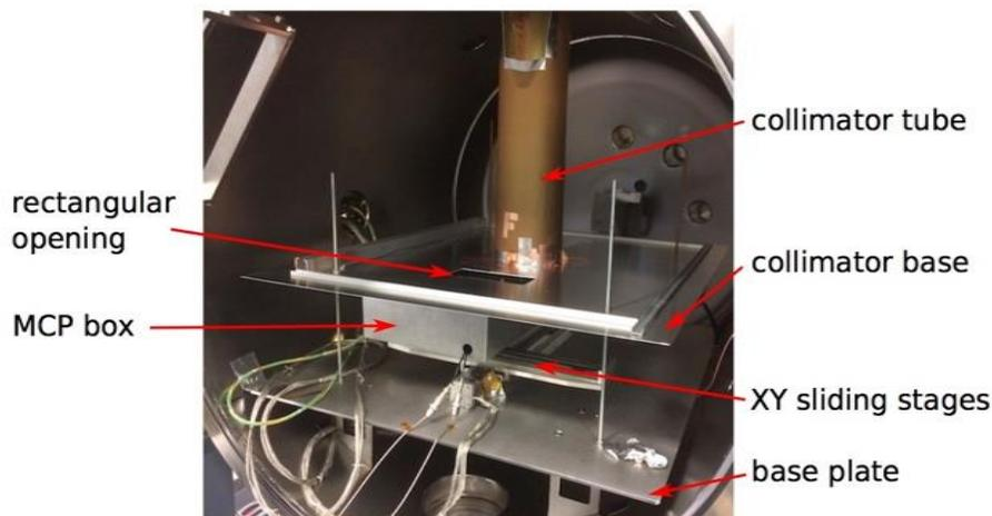
Figure 5. A view on the experimental setup.
