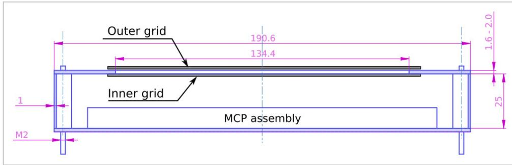
Figure 6. The vertical cut of the MCP box setup.
