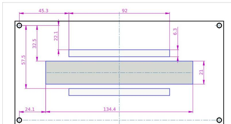
Figure 8. Aperture cover of the MCP box. The dark grey central aperture (STOP sector) is closed by the double mesh. Two light grey apertures (START sectors) are completely opened for UV light.
