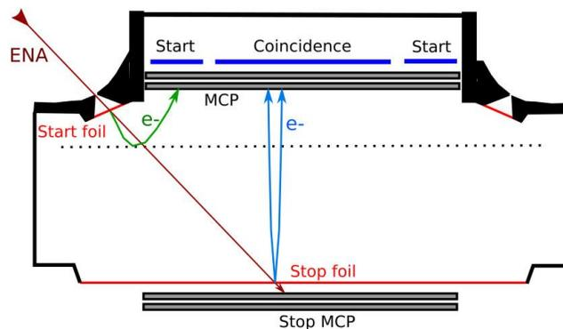
Figure 2. Simplified ENA detection scheme of the JENI instrument
