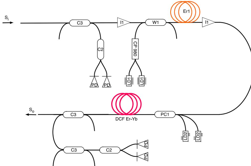
Figure 2: Schematic of the fiber booster amplifier
