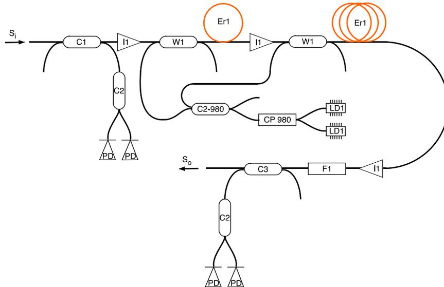
Figure 1: Schematic of the fiber pre-amplifier
