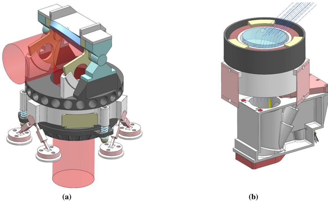
**Figure 7 Two coarse pointing assembly (CPA) architectures TNO is currently developing. (a) A mirror-based configuration targeted for LEO-LEO use-cases. (b) A CPA architecture based on prisms following the Risley-principle which is targeted for LEO-Ground use cases.**
