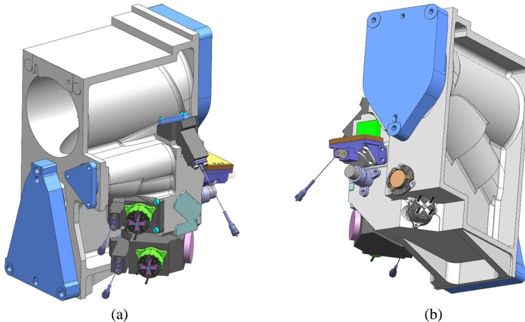
**Figure 3 Preliminary design of a LEO communication terminal with 70 mm entrance aperture front side (a) and back side (b).**
