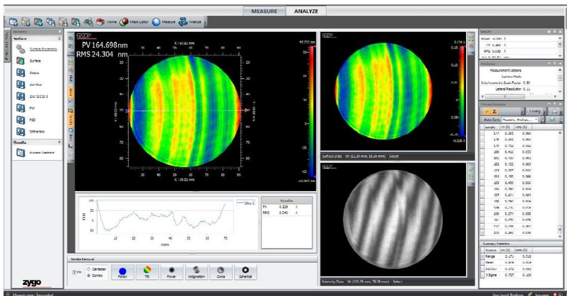
Figure 5 RMS WFE of prototype telescope.
