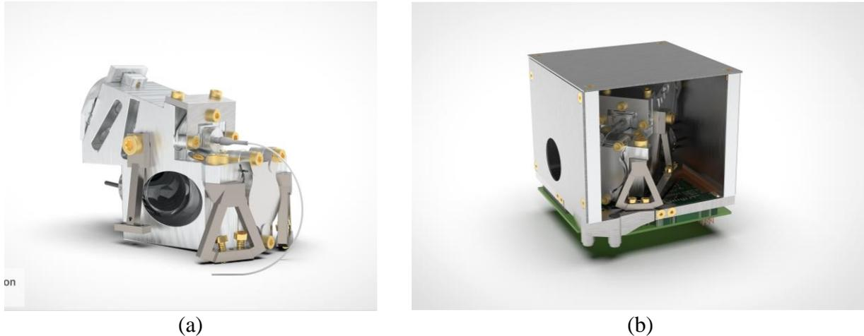
Figure 6 (a) CAD render of the optical bench (b) cad rendering of the optical bench in an cubecat structure
