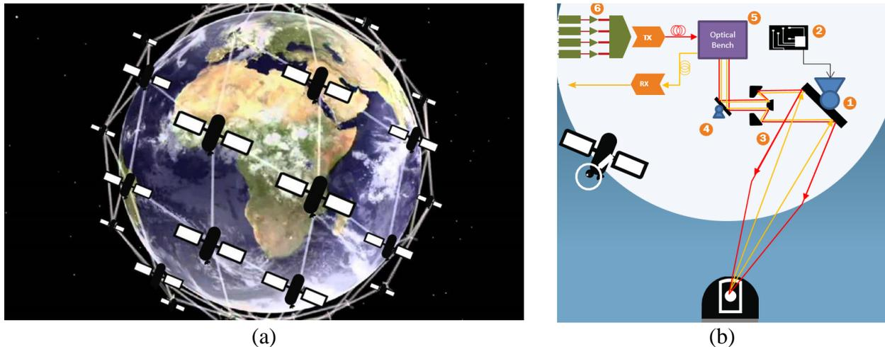
**Figure 1 (a) Massive satellite constellation to connect people everywhere at every time at a reliable and secure way, with low latency. (b) Optical terminal system architecture, with (1) CPA, (2) Controller, (3) Telescope, (4) FSM, (5) Optical Bench, (6) Photonics.**
