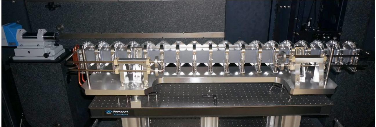
Figure 3. The Diamond NOM slope measuring profiler measuring a large and heavy, side-cooled mirror system.
