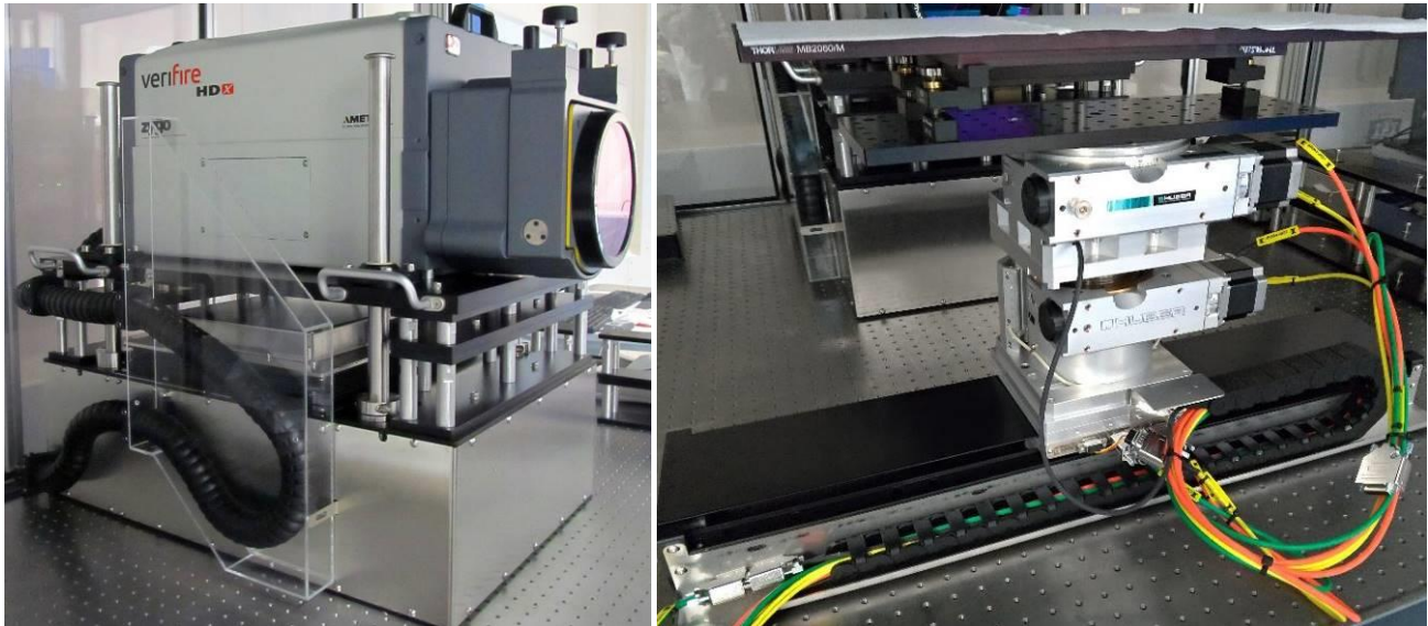
Figure 5. (a) Zygo Verifire 6'' HDX Fizeau interferometer mounted on an in-house-built, modular support platform. (b) Motorized stages for the HDX stitching system which precisely translate and rotate the test optic in front of the Fizeau's beam. A motorized roll stage will soon replace the current manual adjuster.
