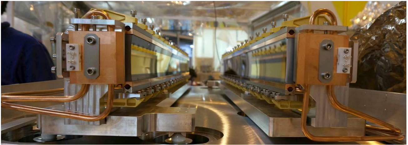
Figure 2. An in-house designed, double toroidal mirror system with side cooling, as installed on the beamline.
