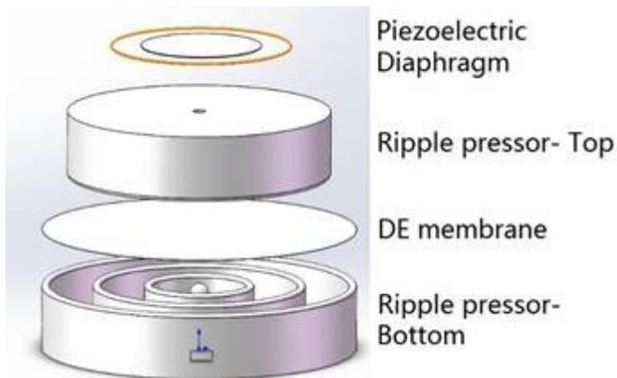
Figure 20: The demo of dielectric elastomer energy harvester autonomously primed by piezo- and tribo-electricity
