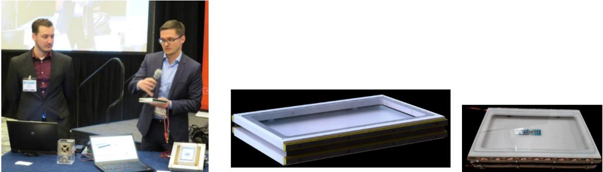
Figure 18: Haptic feedback demonstrators based on strip dielectric elastomer actuators
