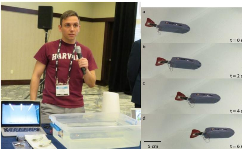
Figure 12: An untethered swimming robot powered by dielectric elastomer actuators
