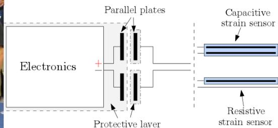
Figure 8: The demonstration of the Capacitive coupling as an underwater signal transmission interface
