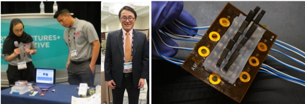
Figure 15: the demo of multiple mode ionic polymer-metal composite array for the use in travelling wave actuators and sensing
