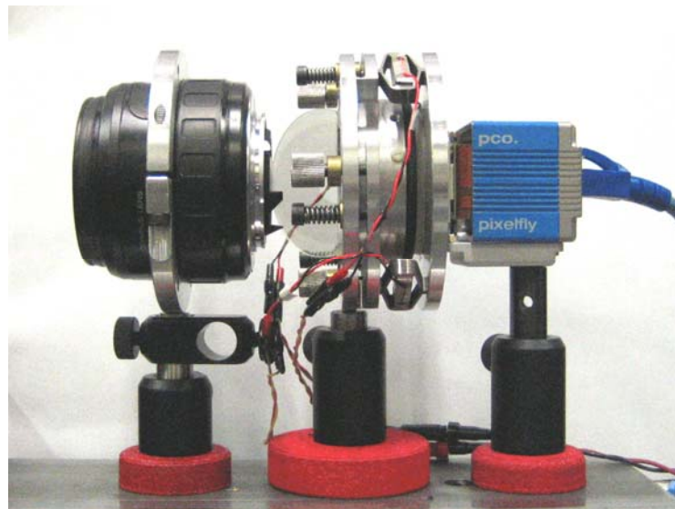
Fig. 1. Picture of the hyperspectral imaging device. From the left: the photographic objective, the F-P interferometer and the monochromatic CCD camera.
