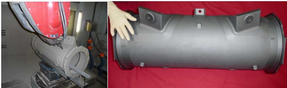
Fig. 2. One of the 19 GAIA torus segments left ) during green machining, right ) ready for brazing assembly
