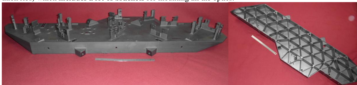
Fig. 6. Views of the BAM large base-plate (0.92 m x 0.28 m - only 5.6 kg)
