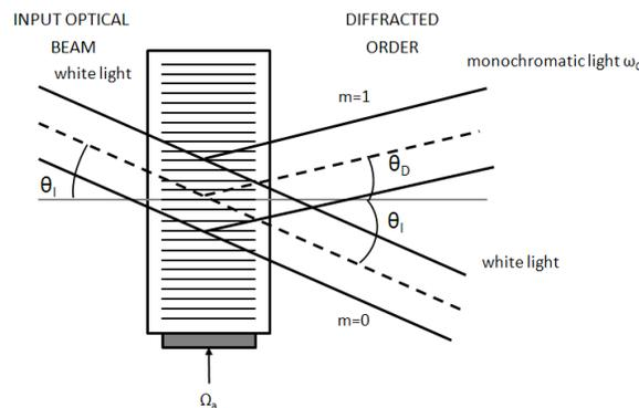
Fig. 3. AOTF concept. When a sine ultrasonic acoustic wave is applied to the crystal, a monochromatic light ( $1^{\text{st}}$  order) exits the crystal in a given direction, distinct from that of the non diffracted white light ( $0^{\text{th}}$  order).
