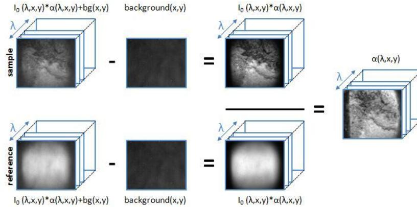
Fig. 2. MicrOmega protocol to get reflectance spectra
