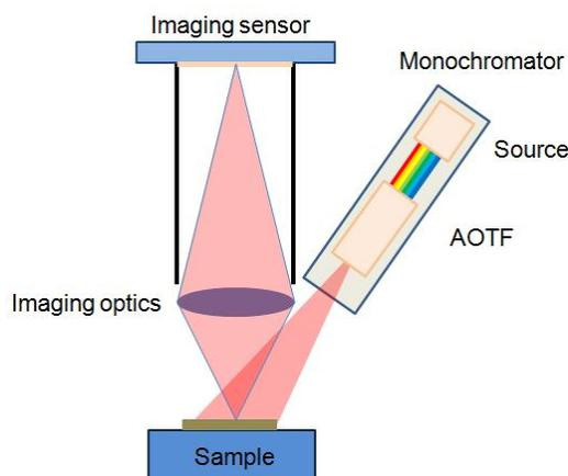
**Fig. 1.** MicrOmega concept diagram with its subsystems: monochromator, imaging optics and imaging sensor.
