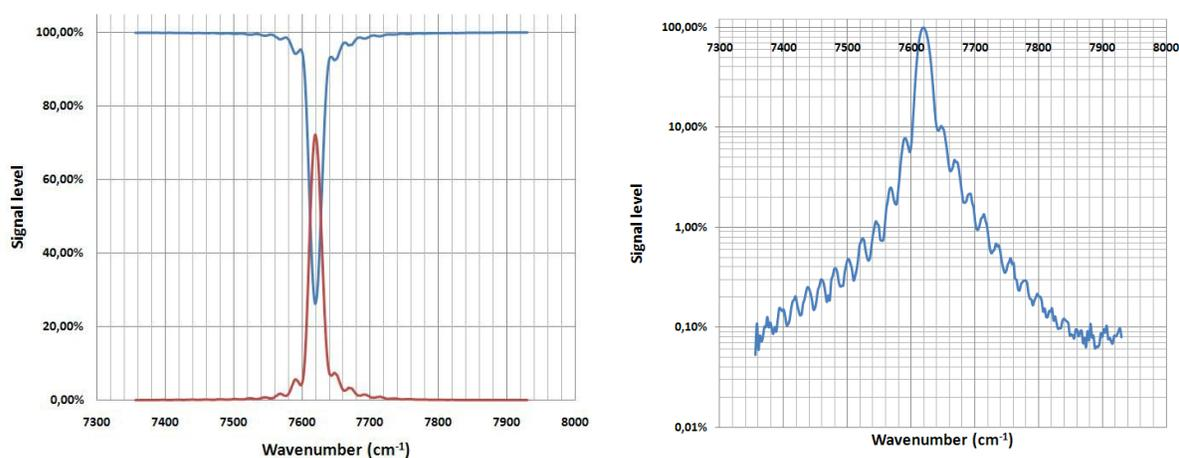
**Fig. 4.** On the left: 0<sup>th</sup> order in blue and 1<sup>st</sup> order in red. About 74% of the 0<sup>th</sup> order is converted to the 1<sup>st</sup> order at the center frequency with a RF power of 1.58 W. On the right: 1<sup>st</sup> order signal level (log scale).
