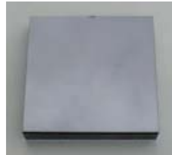
Fig.4 Mirror surface after the third polishing (the direction of the mirror is the same as in Fig.3)
