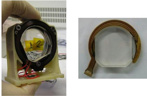
**Fig. 4.** Structural and Thermal Model (STM) of the SO/PHI PMPs. Left, the STM PMP integrated; right, cell with flexible cable including the temperature sensor.
