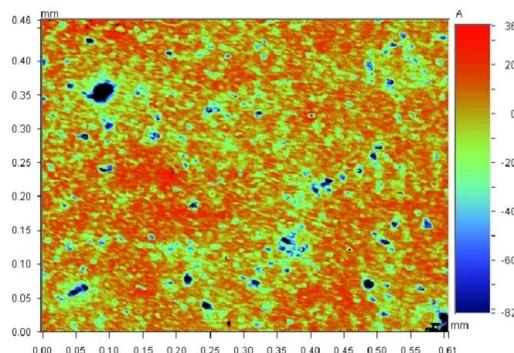
Figure 1 : Example of micro-roughness for NTSIC substrate - 1.5-nm RMS, field 500µm
