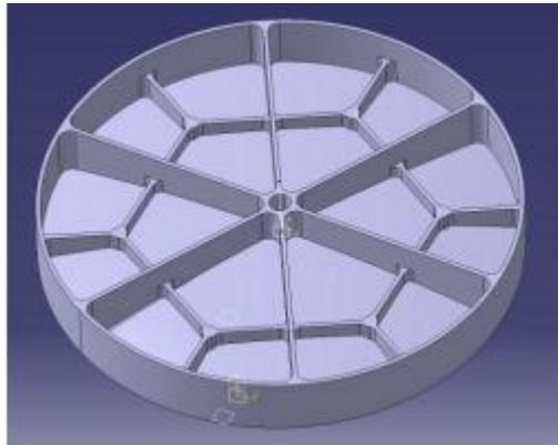
Figure 7 :Design of the mid-size mirror
