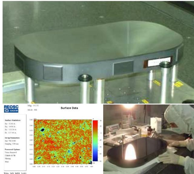
Figure 5 : NTSIC substrate - 1.5-nm microroughness measurement – The polished M3 MSS mirror
