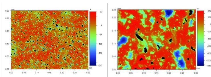
Figure 6 :Boostec SiC polishing (3 nm RMS) / ECM HB-Cesic polishing (30 nm RMS)
