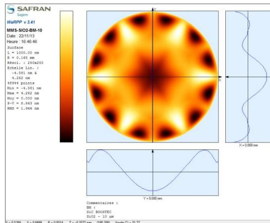
Figure 8 : Distortion at cryo : 2 nm RMS surface error (focus removed) (FE computation)
