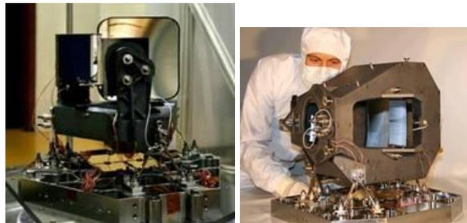
Figure 3 : NIRSpec COL and CAM TMA
